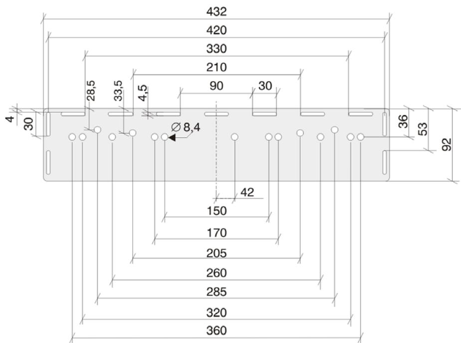
Figure 69: Distances entre les orifices du support type MT-1
