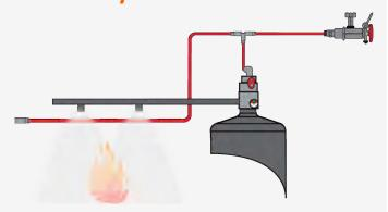
In the indirect system, the sensor tube functions only as a temperature detector. For a correct installation it is necessary to calculate the pipe network.
