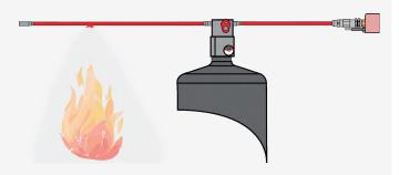
In the direct system, the sensor tube works as a temperature detector and as a network of discharge pipes.
