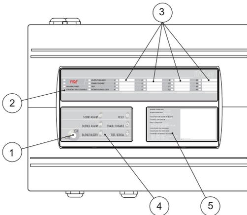
① - Switch for changing over between Access Levels 1 and 2. In **OFF** position (**Access Level 1**) only the **SILENCE BUZZER** button is active and in **ON** position (**Access Level 2**) all buttons are active.
