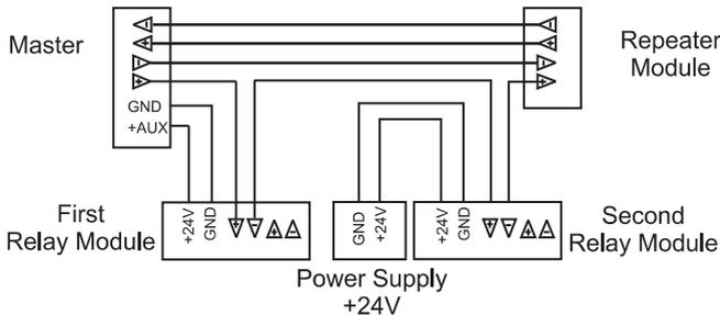
Figure 22. Connecting between two Relay Modules, Repeater and Master Panel.
